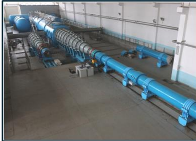
Figure 6 – CAS IOM JF-12 Shock Tunnel, Duplicating Hypersonic Flight Conditions at Mach 5 – Mach 9 288
